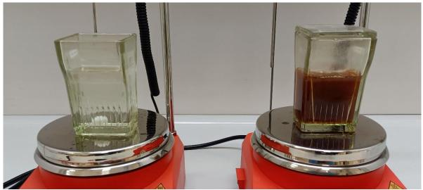
Fig. 4. Laboratory set-up for the slide stain experiment including mixing. On the left, there was 30% H<sub>2</sub>O<sub>2</sub>, and on the right, there was Fenton's solution. Two slides, each with applied samples, were placed in both containers
