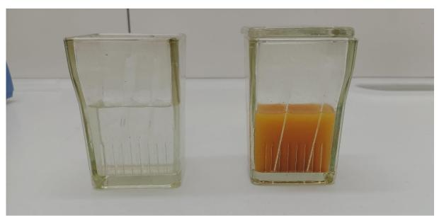
Fig. 3. Laboratory set-up for the slide stain experiment. On the left 30% H<sub>2</sub>O<sub>2</sub>, on the right Fenton's solution. Two slides each with samples applied in both containers
