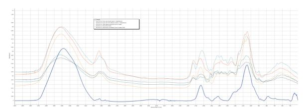
Fig. 2. FT-IR spectrum and spectral database fit factor indicating 97.15% similarity to polyethylene (Primpke 12)
